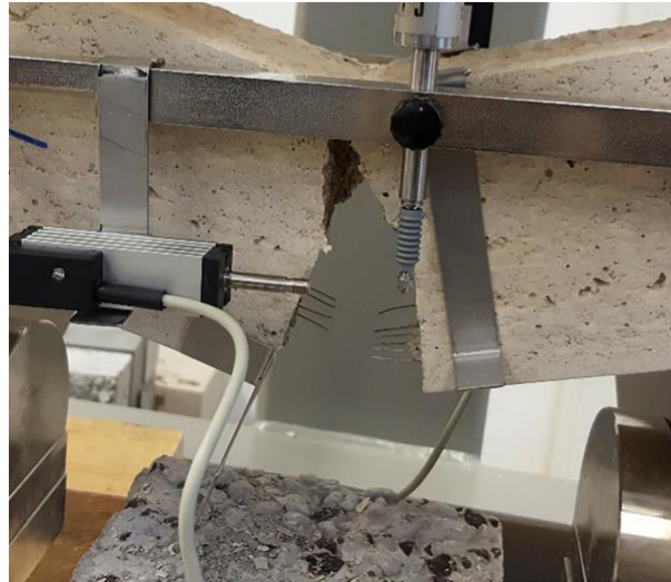
Fig. 1. Three-point bending of a FRC beam.
