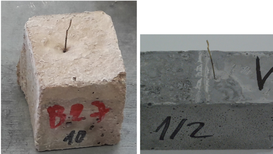
Fig. 2. Concrete samples for fiber for pull-out, left) old sample - fiber inserted after casting, right) new sample - fiber inserted before casting.
