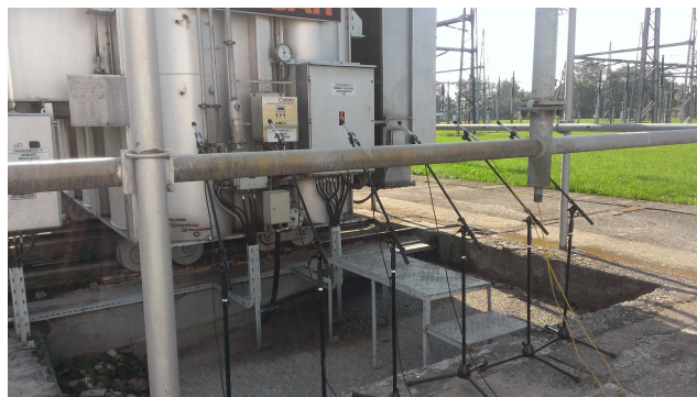
FIGURE 6. Field setup of condenser microphones for recording the OLTC audio signature.
