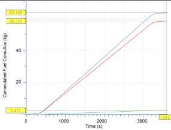
**Figure 9: Cumulated fuel reduction due to the external power supply for auxiliary demand during the voyage**
