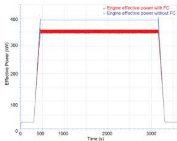
**Figure 8: Engine power reduction due to the external power supply for auxiliary demand during the voyage**
