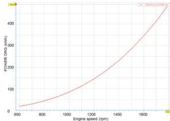
Figure 1: Propeller curve
