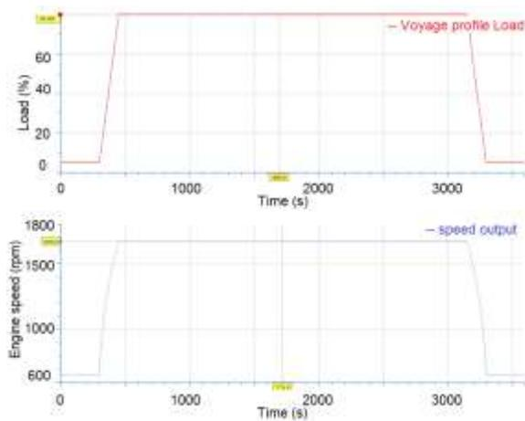
**Figure 6: Engine speed and load profile during 1 hour voyage**
