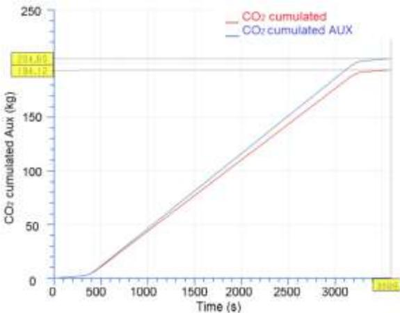
**Figure 10: Cumulated CO<sub>2</sub> reduction due to external power supply for auxiliary demand during the voyage**
