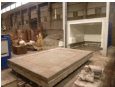
Figure 1. Refractory prototypes produced at industrial scale for validation at the demo site of the ceramic sector
