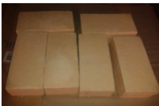
Figure 1. Refractory prototypes produced at industrial scale for validation at the demo site of the ceramic sector
