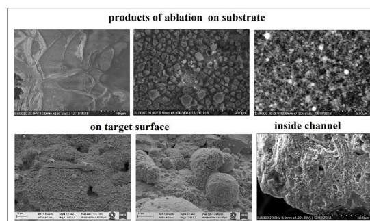
Fig. 2. SEM micrograph of ablation products precipitated on the substrate, the surface of ceramics and formed inside the crater.
