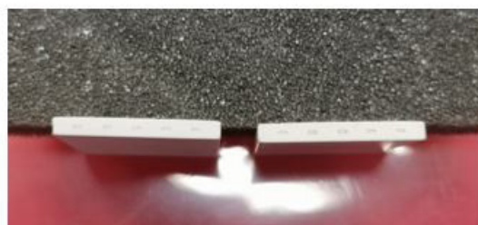
After printing and cutting the part, we can observe the internal cannel made with polymerized resin
