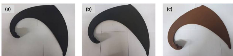
Fig. 2. Ceramic cores prepared using the 3D printer and inorganic binder: (a) BJ type (USA, E company), (b) BJ type (German, V company), and (c) SLS type (Korea, S company).
