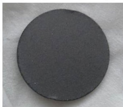
b) GaV 4 S 8 ceramic target (20 mm in diameter)
