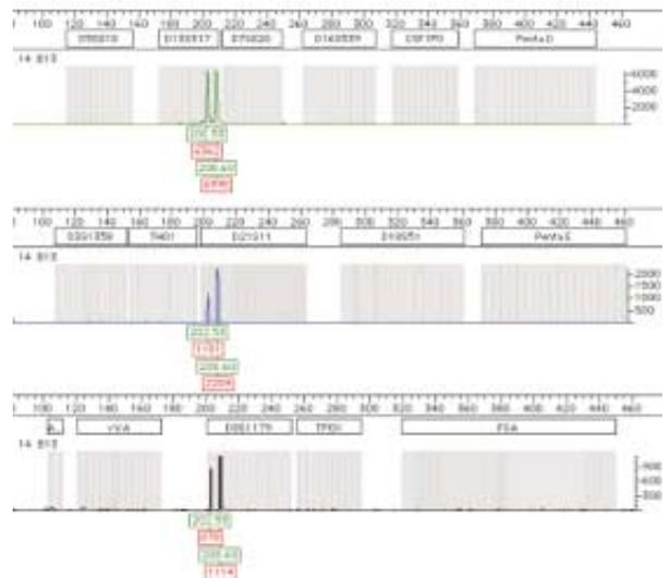
**Figure 12.** The 202 and 208 green products (shown in the upper row of picture) and blue and yellow pull-up (shown in the middle and the bottom row, respectively) observed after PCR amplification with PowerPlex™ 16 kit of genomic DNA from the yeast *Rhodotorula glutinis*.
