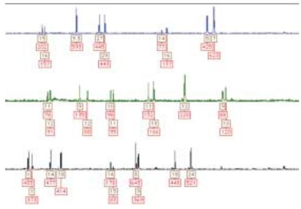
**Figure 3.** Multilocus STR profile obtained with PowerPlex™ 16 kit from a DNA sample isolated from an 8-year-old bone sample with no detectable amounts of nuclear human DNA. Note the extensive dropout of some alleles.
