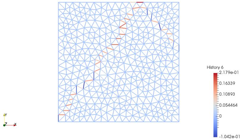
Figure 5: Final cracks formed after compression test
