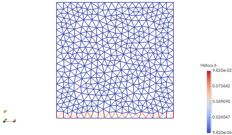
Figure 3: Final cracks formed after tension test
