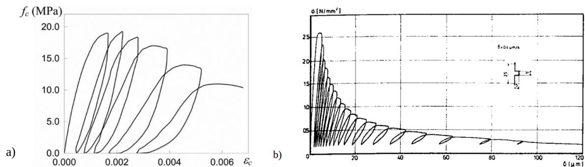
Figure 1: Cyclic compression test a) from Karsan and Jirsa (1969) and cyclic tension test b) from Reinhardt (1984)
