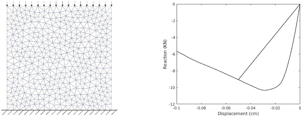
Figure 4: Uniaxial compression test: a) mesh and b) computed macroscopic response
