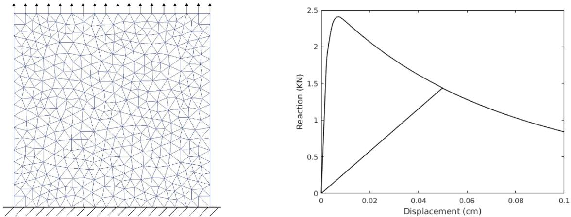
Figure 2: Uniaxial tension test: a) mesh and b) computed macroscopic response
