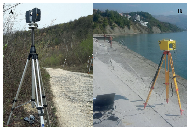
Fig. 1 a) Faro Focus X 130 terrestrial laser scanner at Bizek quarry; b) Optech ILRIS 3D scanning coastal cliff at Duilovo
