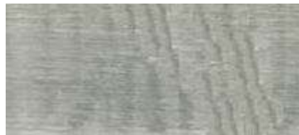
Figure 3. Luders bands on the surface of cold drawn pipe of niobium microalloyed steel
