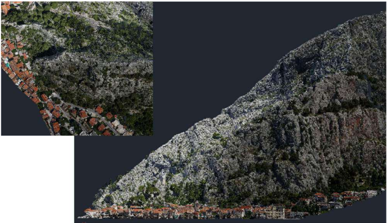
Figure 3 3DPC provided by TLS and SfM techniques. A view at the slope (down); a layout over the middle part of the town (left up).
