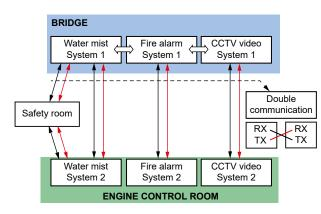
Figure 2. Display of high redundancy, according to SOLAS regulations, for safe return to the port
