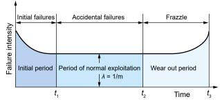
Figure 1. Fault intensity function
