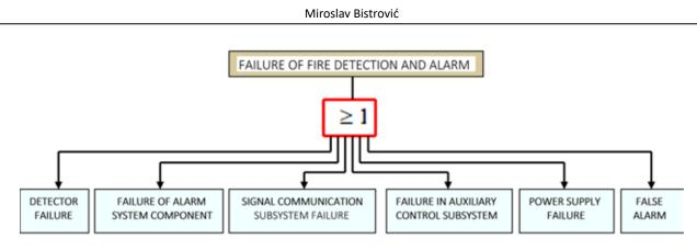
Figure 3. Map of fault detection and fire alarm divided into six subsystems
