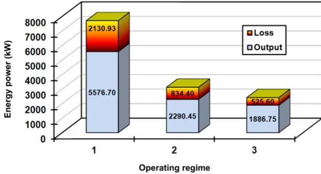
Fig. 2. Change in energy power output and energy power loss of the analyzed deaerator in three operating regimes
