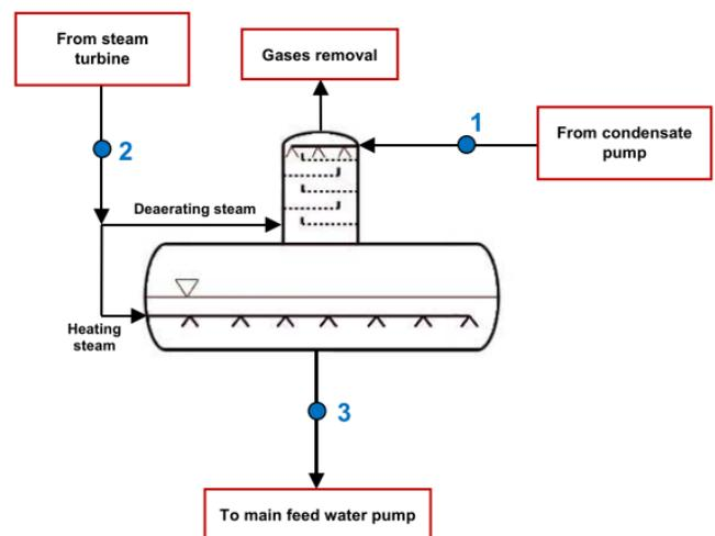
Fig. 1. Main scheme and required operating points of the analyzed deaerator
