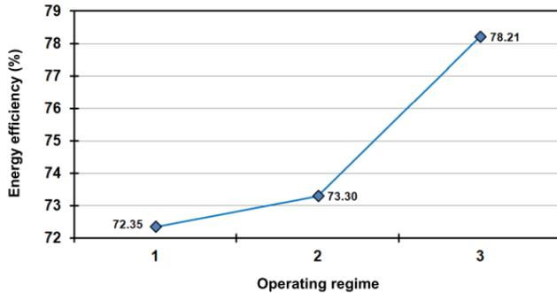
Fig. 3. Change in energy efficiency of the analyzed deaerator in three operating regimes
