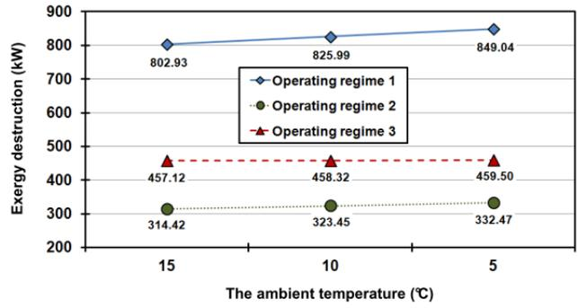
Fig. 4. Change in the exergy destruction of the analyzed deaerator in three operating regimes and at three ambient temperatures
