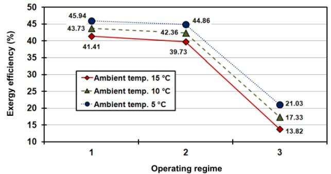
Fig. 5. Change in exergy efficiency of the analyzed deaerator in three operating regimes and at three ambient temperatures
