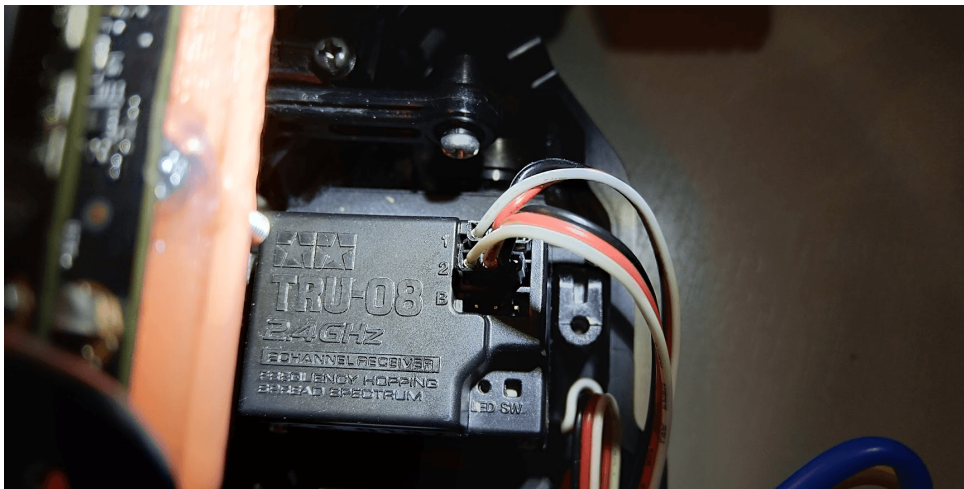
Figure 38: The RC car receiver with ESC and servo connectors
