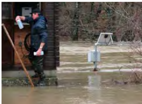
Figure 5. Sampling with a milk bottle on the Reka River (Photo: Ulaga, F.)
