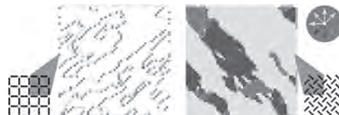
Magnetization maps of square (right) and pinwheel (left) ASI. Each pixel represents the net magnetization of eight magnets, highlighted in insets. Note that white indicates no net magnetization (the eight moments cancel).
