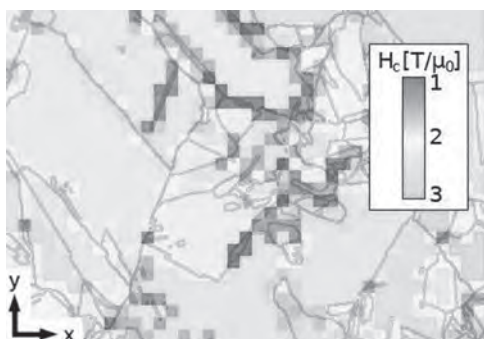
Fig. 1: Local nucleation fields for subsets (color coded squares) of magnetic sample with microstructure shown in background.
