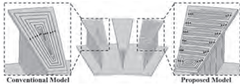
Theoretical conventional AFPMSM and proposed AFPMSM eddy current loss loop
