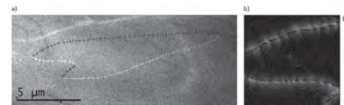
Fig. 2: (a) LTEM image of a saw-tooth domain (b) Induction map showing the in-plane magnetization profile of the leftmost section of the domain as calculate using the transport-of-intensity equations formalism.
