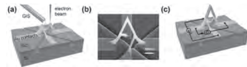
Fig.1 Direct fabrication and measurement of the Co nanobridge
