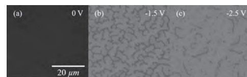
Fig. 2: MOKE images of domain structures of MgO/ Mn 2 CoAl/ Pd trilayers captured with H_z = -1 mT at 0, -1.5, -2.5 V, respectively.
