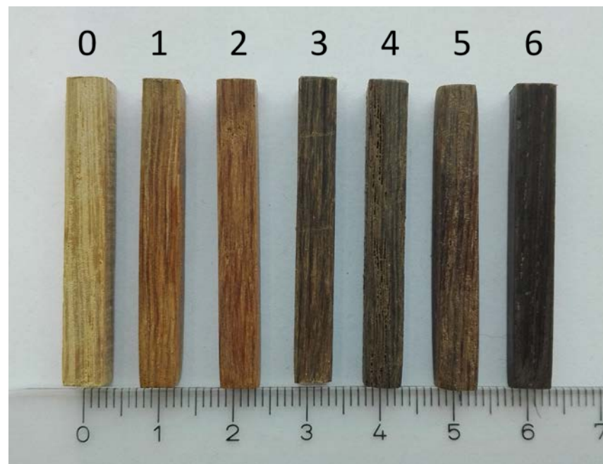
Figure 2. Wood specimen prepared for the abrasion testing arranged from the recent oak (0) to the oldest subfossil oak (1–6).
