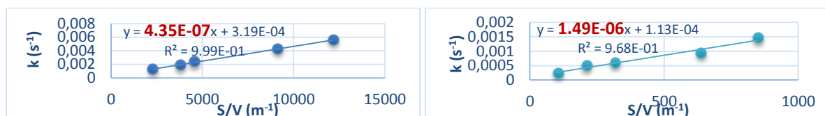
Figure 1. First-order rate constant k ( \text{s}^{-1} ) as a function of solid surface area over total solution volume ratio [S/V ( \text{m}^{-1} )] for different amounts of UC (left) and UN (right) in 25 mL 10 mM \text{NaHCO}_3 solution after exposure to 0.2 mM \text{H}_2\text{O}_2 .
