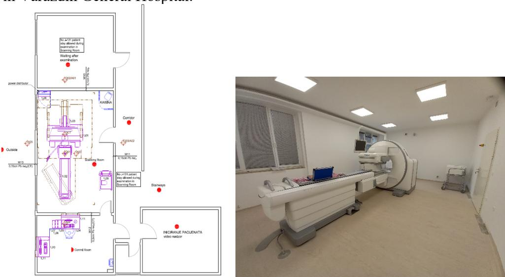
Figure 1: a) Floor plan for the diagnostic block where SPECT/CT scanner was eventually installed;
