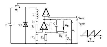
Fig.1. Functional diagram of the buck converter
