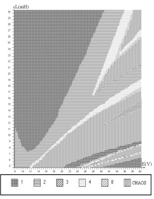
Fig.5. Input voltage vs. load inductance (*EL*) bifurcation diagram (*T*=330μs) representing zones of period-*N* operation and chaos (*N*=1,2,3,4,8)
