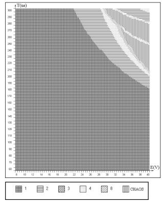
Fig.6. Input voltage vs. period of the external sawtooth ramp voltage (*ET*) bifurcation diagram (*L*=15mH) representing zones of period-*N* operation and chaos (*N*=1,2,3,4,8)
