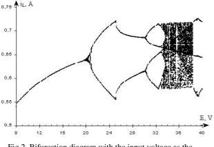
Fig.2. Bifurcation diagram with the input voltage as the bifurcation parameter (*L*=15 mH, *T*=330µs, ∠*E*=0.1V)
