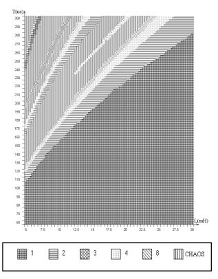
Fig.7. Load inductance vs. period of the external sawtooth ramp voltage (*LT*) bifurcation diagram (E=22V) representing zones of period-*N* operation and chaos (N=1,2,3,4,8)
