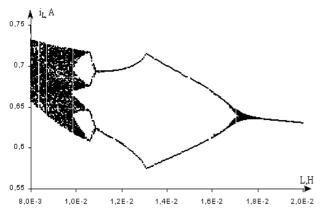
Fig.3. Bifurcation diagram with the load inductance as the bifurcation parameter (E=22V,  $T=330\mu s$ ,  $\Delta L=50\mu H$ )
