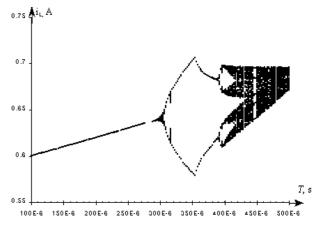
Fig.4. Bifurcation diagram with the period of external sawtooth ramp voltage as the bifurcation parameter (E=22V, L=15mH,  $\Delta T=1\mu$ s)
