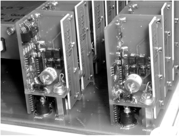
Figure 4. Picture of realized protection circuits.
