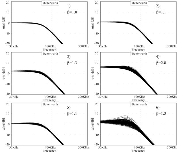
Fig. 11. Passive components Monte Carlo runs of amplitude response of capacitively-tapered 4<sup>th</sup>-order LP filter as a function of  $\beta$  (Table IV).
