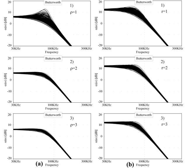
Fig. 4. Passive components Monte Carlo runs of impedance-tapered 4<sup>th</sup>-order LP filters as given in Table II. (a) Capacitively. (b) Resistively.
