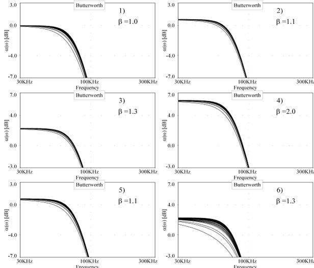
Fig. 12. Active component (opamp) MC runs of amplitude response of capacitively-tapered 4<sup>th</sup>-order LP filter as a function of  $\beta$  (Table IV).
