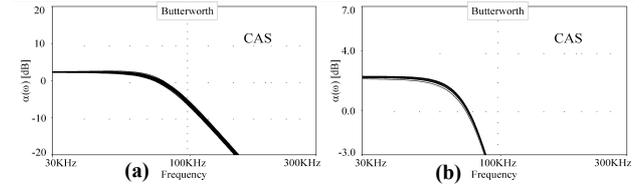
Fig. 14. (a) Passive, and (b) active sensitivity represented by MC runs of amplitude response of CAS 4<sup>th</sup>-order LP filter (Table V).
