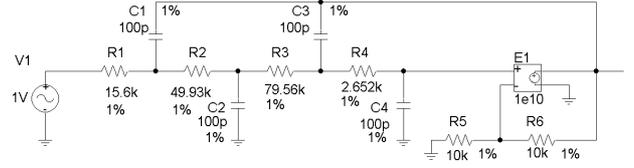
Fig. 3. PSpice circuit model of 4<sup>th</sup>-order LP filter for *passive* components MC runs.
