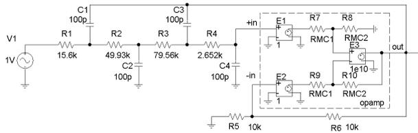
Fig. 7. PSpice circuit model for an active component MC runs.
