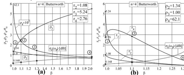
Fig. 13. Design parameters in Table IV as a function of  $\omega_0$ . Note that the abscise-axis is represented by  $\beta$ . (a) R-Tapering. (b) C-Tapering.
