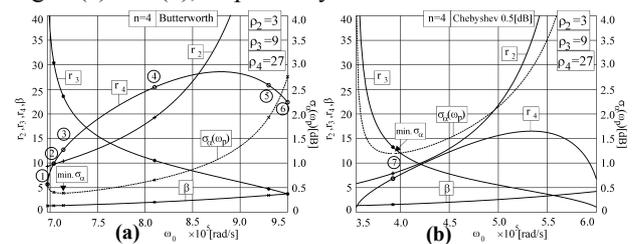
Fig. 5. Design parameters  $r_2$ ,  $r_3$ ,  $r_4$  and  $\beta$  in Table III as a function of  $\omega_0$ .
