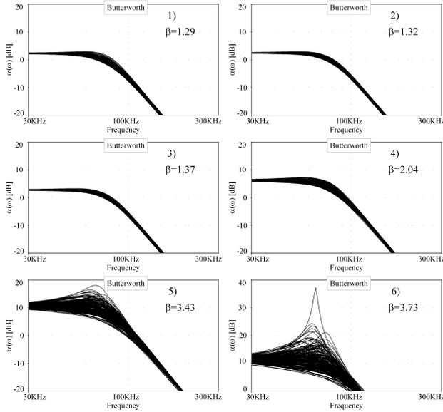
Fig. 6. Passive components Monte Carlo runs of amplitude response of capacitively-tapered 4<sup>th</sup>-order LP filter as a function of  $\omega_0$  (Table III).
