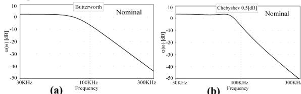
Fig. 2. Magnitude of transfer functions for filters in Table I. (a) Butterworth. (b) Chebyshev with  $R_p=0.5[\text{dB}]$ .
