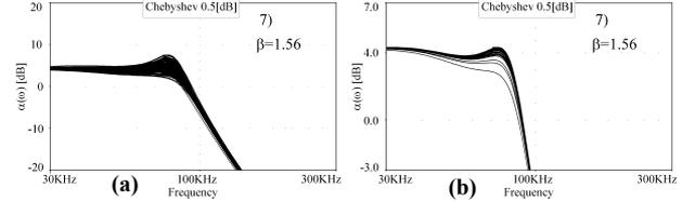
Fig. 10. (a) Passive, and (b) active sensitivity represented by MC runs of amplitude response of Chebyshev filter no. 7) in Table III.
