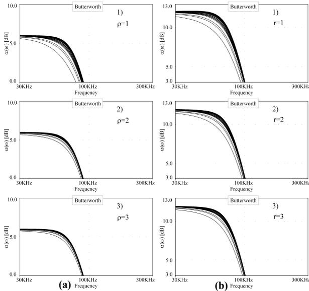
Fig. 8. Active component (opamp) MC runs of impedance-tapered 4<sup>th</sup>-order LP filters as given in Table II. (a) Capacitively. (b) Resistively.
