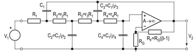
Fig. 1. 4<sup>th</sup>-order LP filter with single opamp and impedance scaling factors  $r_i$  and  $\rho_i$ ; ( $i=2,3,4$ ).
