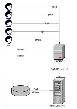
Fig. 4 Scheme of RADIUS architecture of the user's access to the network
