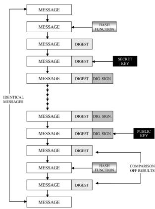
Fig. 10 Principle of functioning of the electronic signature
