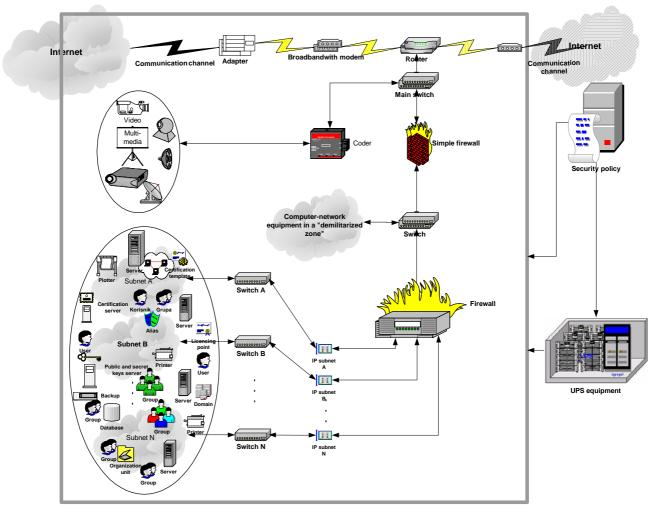
Fig. 2 Physical implementation of network-computer system - model of network security
