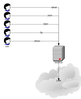
Fig. 3 Scheme of user's access to the network through NAS/RAS server
