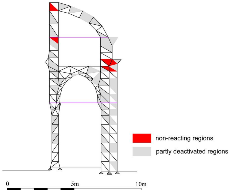
Figure 9: Critical regions in the structure completed up to the upper, semi-barrel vault of the aisles (structure tightened with tie-rods)
