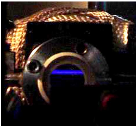
Fig. 6. Blue fluorescence observed at 7P \rightarrow 6S transition in the Cs–He mixture at cesium ground state density N_{Cs} = 3 \times 10^{12} \text{ cm}^{-3} , and He pressure of 12.2 mbar. Photo was taken through the heat-pipe side-window by digital camera.
