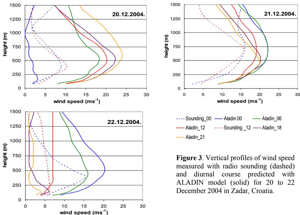
**Figure 3.** Vertical profiles of wind speed measured with radio sounding (dashed) and diurnal course predicted with ALADIN model (solid) for 20 to 22 December 2004 in Zadar, Croatia.
