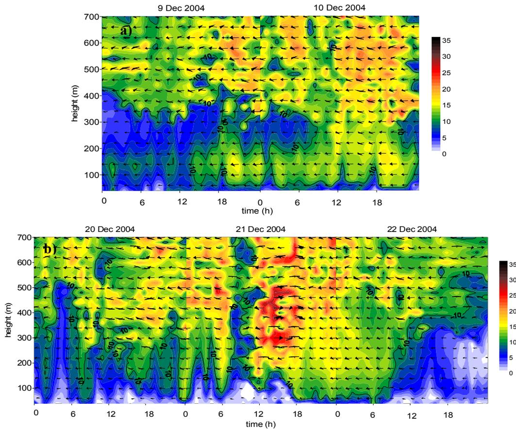
**Figure 4.** Sodar wind speeds and direction measurements for a) 9-10 December 2004 and b) 20-22 December 2004 at Zadar, Croatia.
