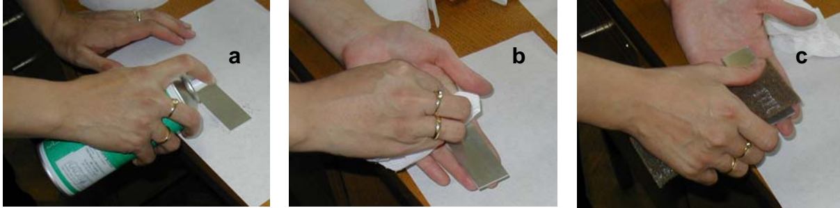
Figure 2. Degreasing (a,b) and grinding (c) of plates
