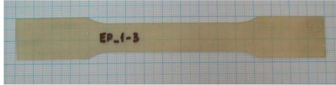
Figure 1: Adhesive tensile test specimen
