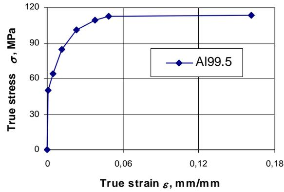
Figure 6: Discretized adherend (aluminium) stress-strain curve
