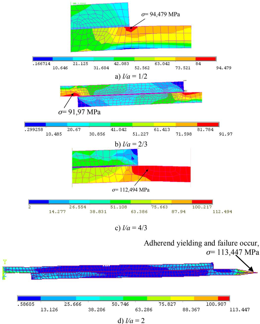
Figure 14: Numerically calculated von Mises stresses in aluminium adherends
