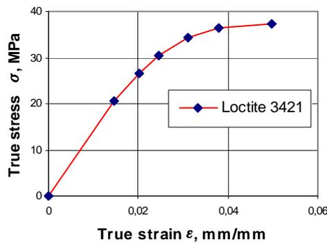
Figure 7: Discretized adhesive (epoxy) stress-strain curve
