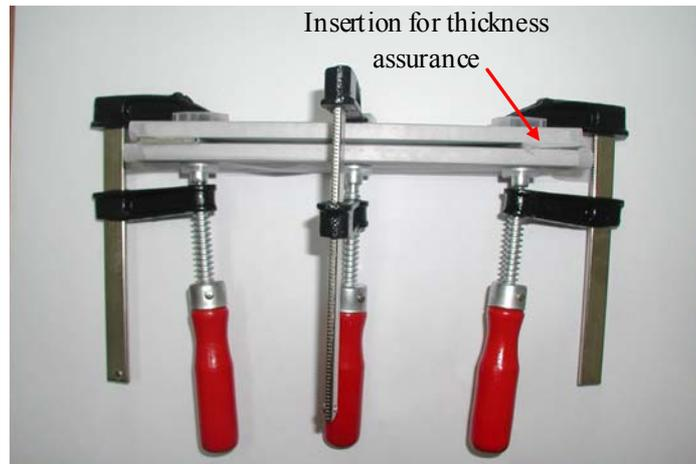
Figure 2: Mould for rectangular specimen production
