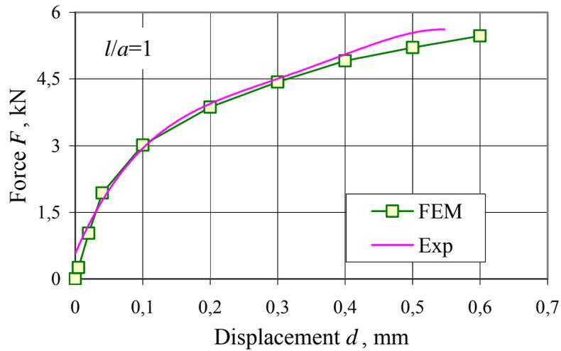
Figure 10: Comparison of experimental and numerical results (relative lap length,  $l/a = 1$ )
