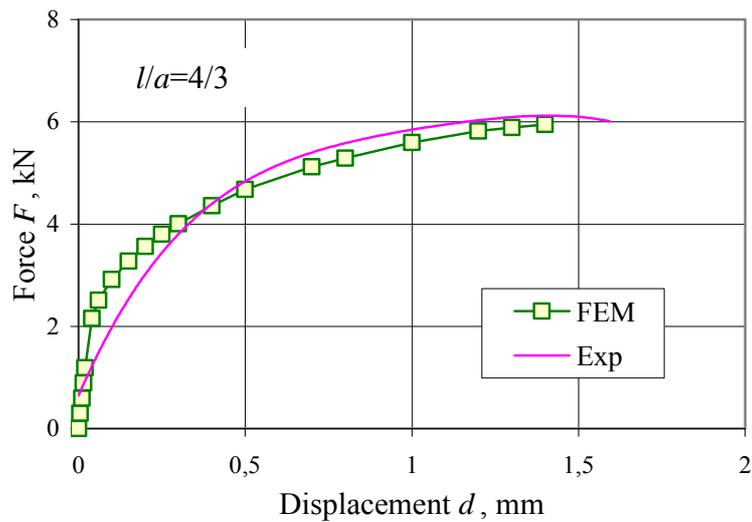
Figure 11: Comparison of experimental and numerical results (relative lap length,  $l/a = 4/3$ )
