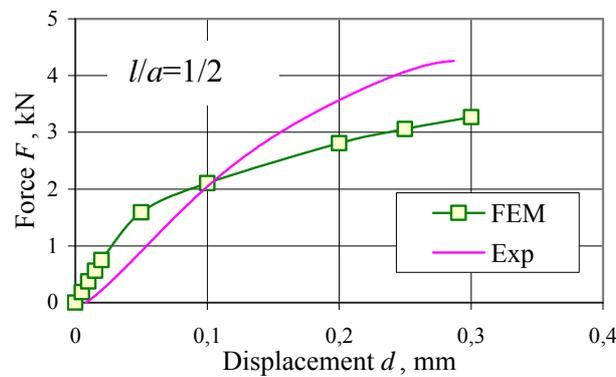
Figure 8: Comparison of experimental and numerical results (relative lap length,  $l/a = 1/2$ )
