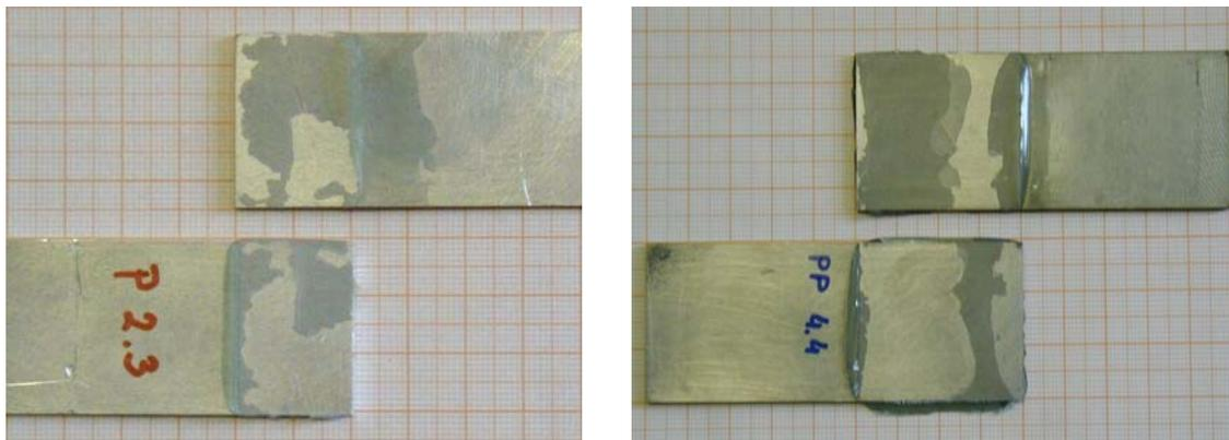
Figure 13: Mixed failure in bonded single-lap joints
