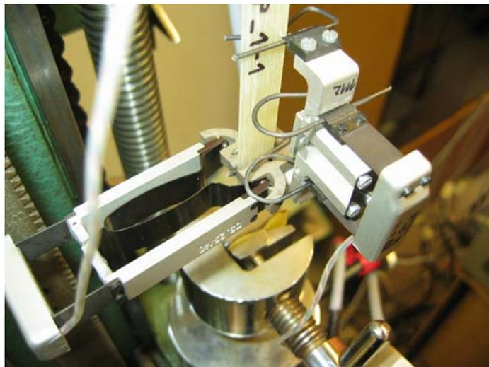
Figure 3: Tensile test of an adhesive specimen
