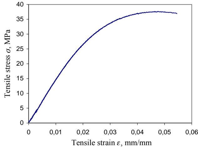
Figure 4: Tensile stress-strain curve of epoxy adhesive
