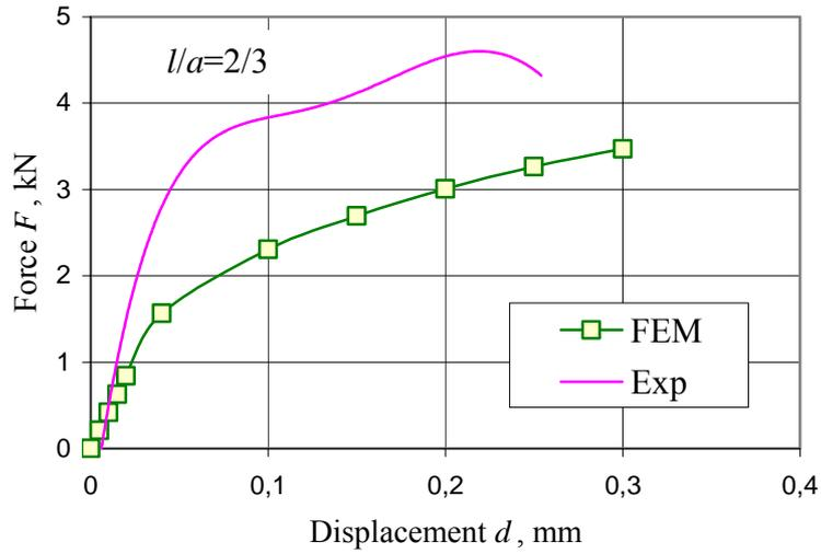
Figure 9: Comparison of experimental and numerical results (relative lap length,  $l/a = 2/3$ )
