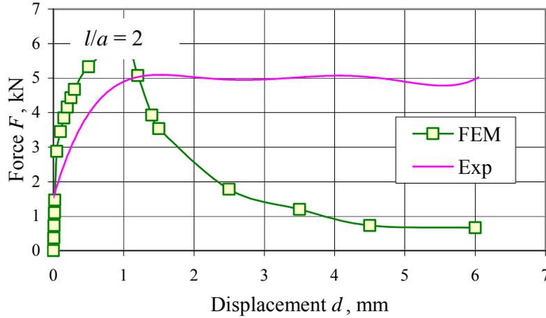
Figure 12: Comparison of experimental and numerical results (relative lap length,  $l/a = 2$ )
