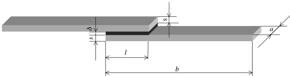
Figure 5: Single lap bonded joint specimen
