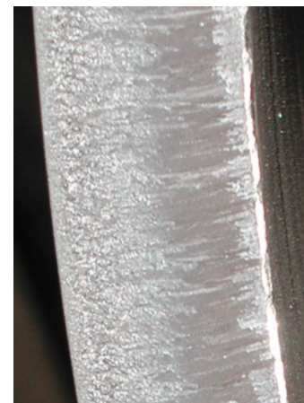
Figure 8. An example of stainless steel air plasma cutting in bellows production process. b) detail of cut surface quality b) welded cylindrical ring after air plasma cutting and cold forming process
