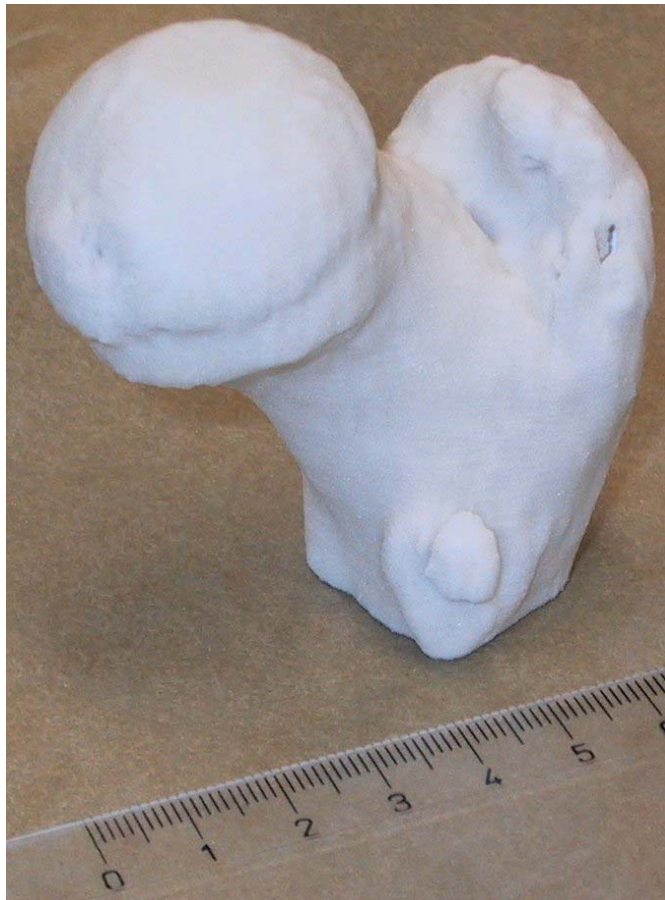
Figure 3. Hip bone shape obtained in 3D printing RP technique
