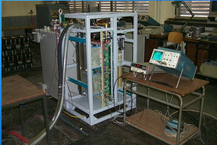
Train heating converter
