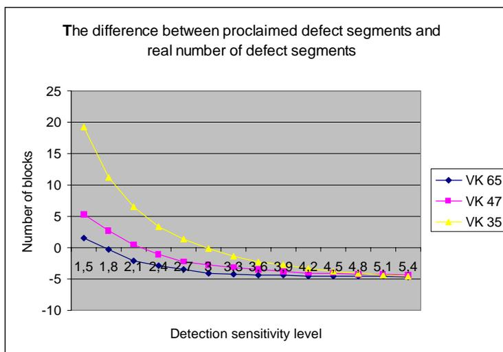
Fig. 5 The difference between proclaimed number of defect segments and real number of defect segments as a function of detection sensitivity level for three segment sizes.
