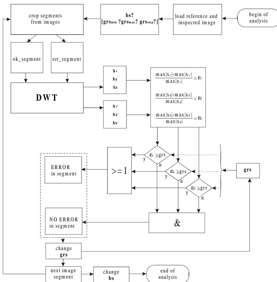
Fig.3 The detailed image processing diagram for Matlab application.
