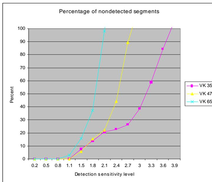
Fig.6 The percentage of nondetected segments as a function of DSL for three block sizes.
