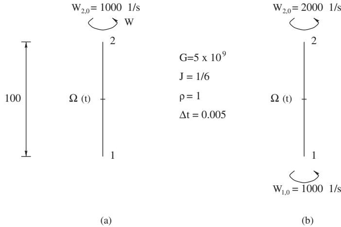
Figure 2. Unsupported rod subject to initial axial angular velocities: (a) only at node 2, (b) at both nodes.
