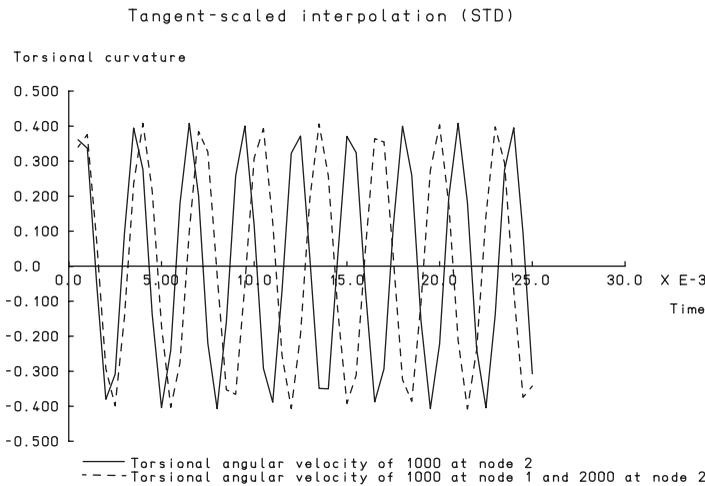
Figure 3. Algorithm (1): Torsional curvature in the centre of the rod in Figure 2: initial conditions (a) (solid line), initial conditions (b) (dashed line).
