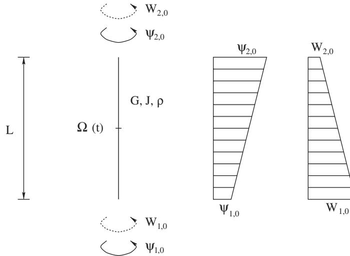
Figure 1. Uniform rod subject to initial rotations and angular velocities at each end.
