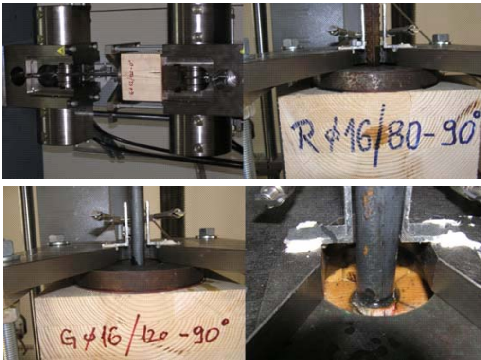
Fig 3: Setting up of experiments with EPOCON 88 glue
