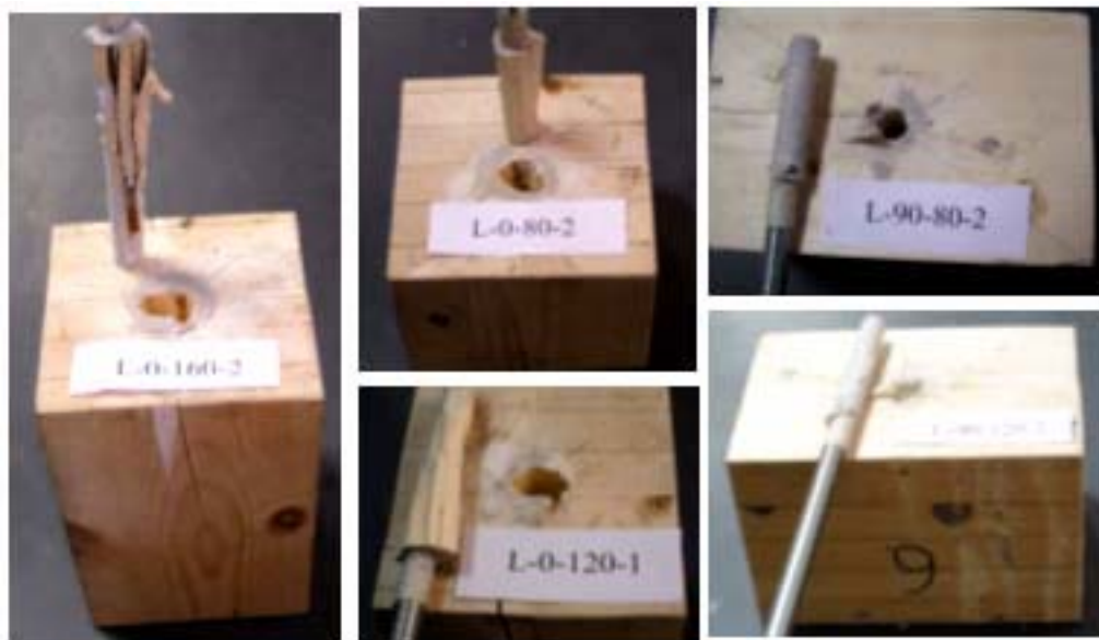
Fig. 4: The two basic types of fracture behaviour for joints with threaded bars due to load angle related to fibers
