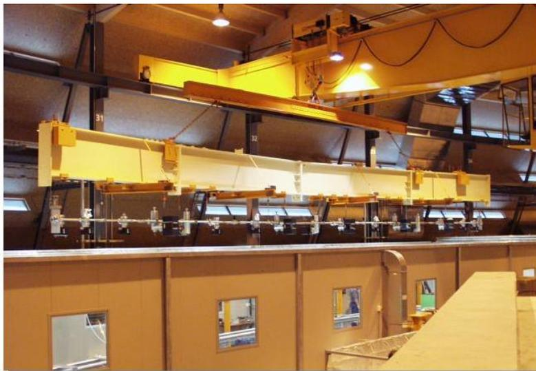
**Fig. 26:** Vacuum chamber transport from the bake-out oven to the storage ring tunnel
