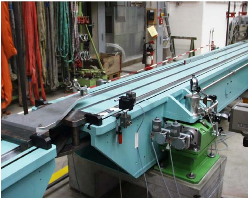
**Fig. 15:** HPS prototype being validated with the laser interferometer
