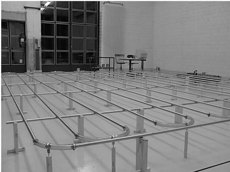
**Fig. 13:** A  $100\text{ m}$  piping HLS experimental set-up
