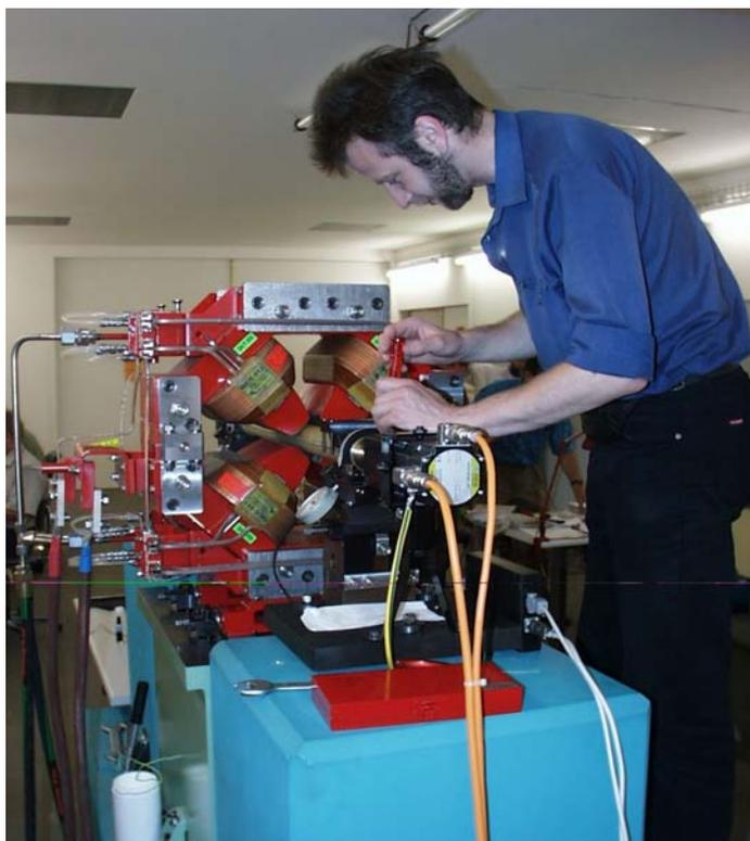
**Fig. 24:** BINP specialist at the SLS rotating coil magnetic measurement bench
