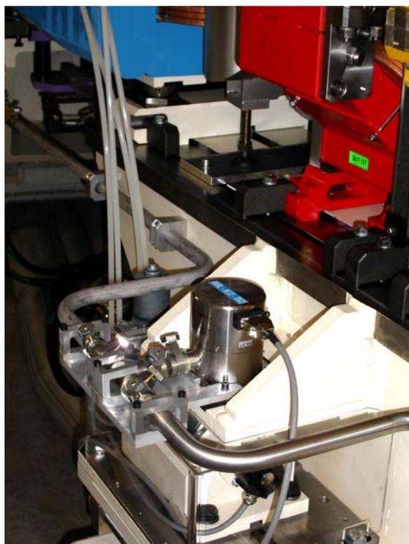
**Fig. 29:** Additional piping fastenings at the HLS pots
