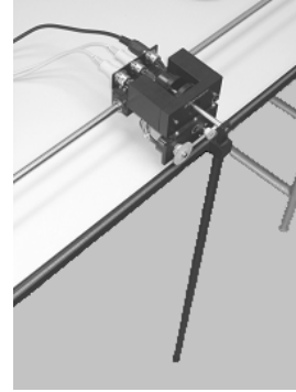
Fig. 7. Single pendulum gantry laboratory model
