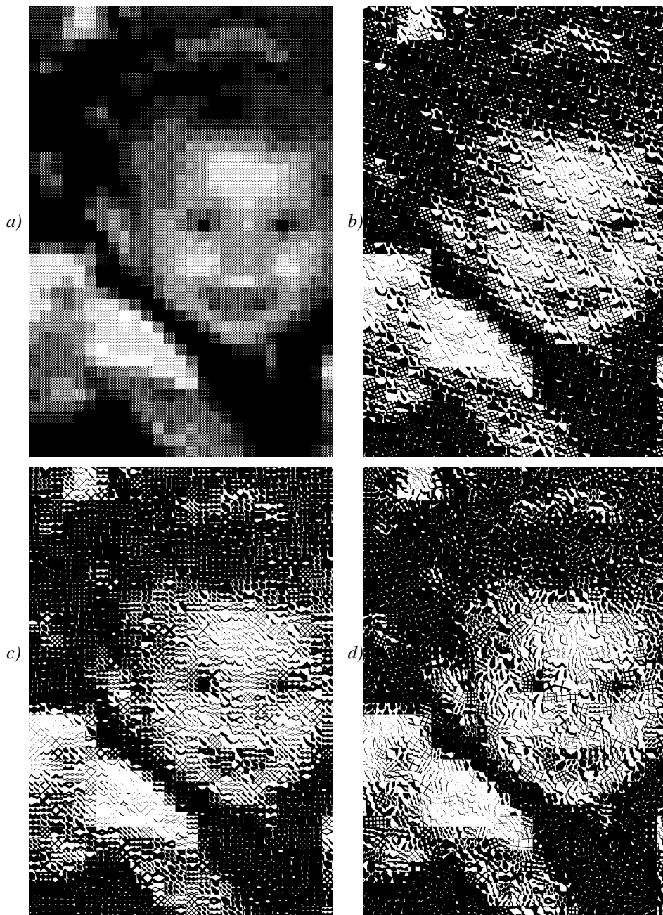
Figure 3. a) standard dot halftone screen b) screening with cyclic continuity of screening algorithm c) screening with stochastic selection of halftone screen element shape algorithm (SEED = 12345678) i \alpha = 0^\circ d) screening with random selection of halftone screen element algorithm and random selection of screening angle \alpha (SEED = 246135)
