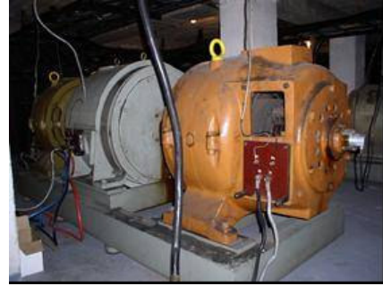
Fig. 4. Synchronous generator with prime mover DC motor
