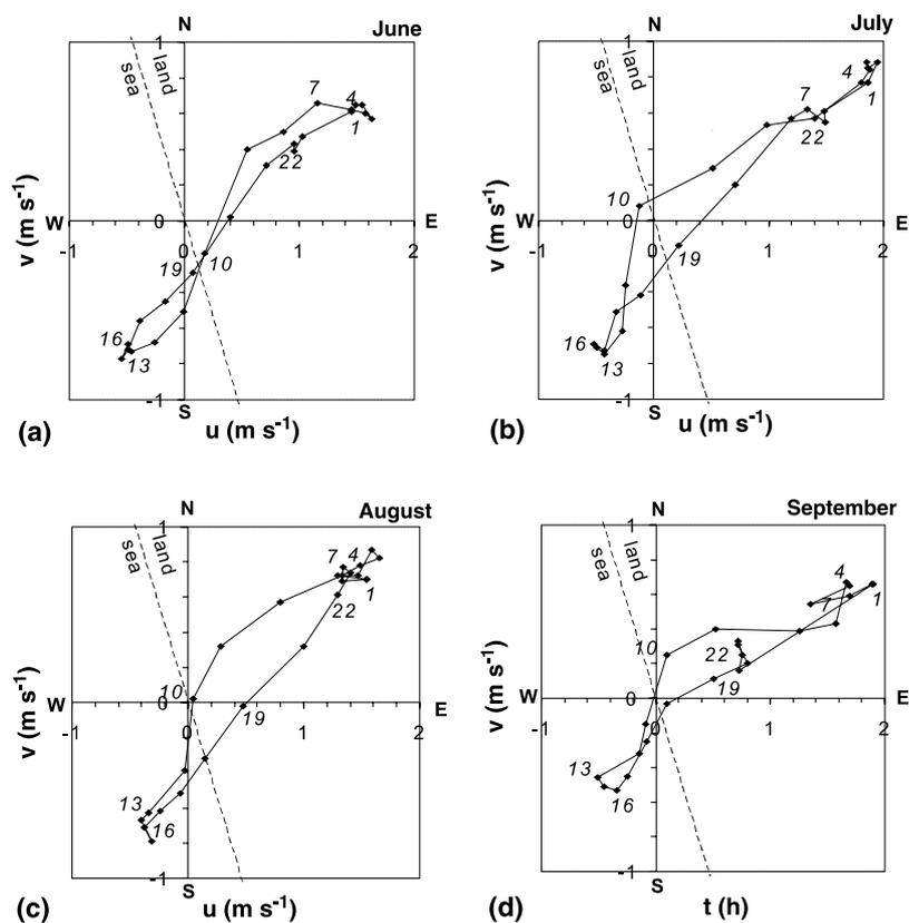
**Fig. 10.** The hodograph of the climatological observed surface wind vectors ( $\text{m s}^{-1}$ ) calculated for the selected SLB dataset for the period 1991–2004 for Senj: (a) June, (b) July, (c) August and (d) September. The wind vectors are directed toward the origin of the coordinate system. Dashed line represents the orientation of the coastline and the numbers represent local time
