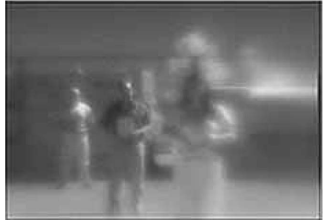
Fig. 4. Image reconstructed by MART algorithm after 50 iterations.
