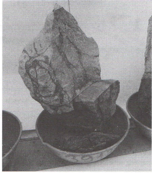
Fig. 13 Capillary rise on the discontinuities of the specimen. The specimen is partially submerged
