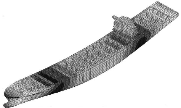
Figure 1: Typical structural mesh.
