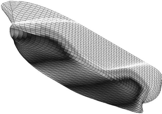
Figure 7: *Nonlinear pressure distribution.*
