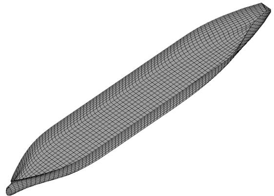
Figure 2: Typical hydrodynamic mesh.
