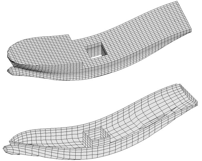
Figure 6: *First bending mode on the structural mesh (above) and its projection on hydrodynamic mesh (below).*
