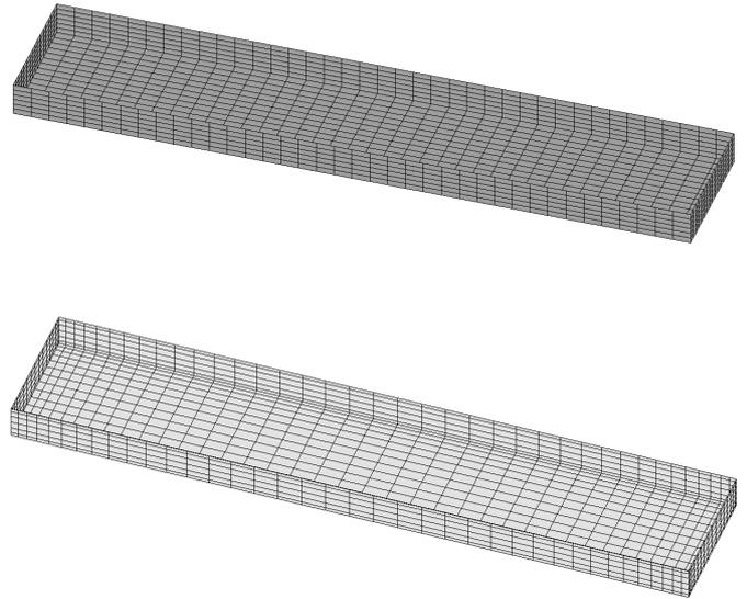
Figure 4: *Hydrodynamic models of the barge. Top - hydrodynamic mesh identical to the structural mesh, bottom - hydrodynamic mesh different from the structural mesh.*
