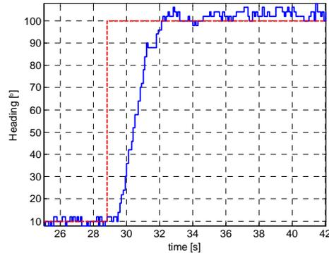
**Figure 4:** The result of the autotuning procedure on the improvement of course servo-control on a cheap, commercially available micro-ROV VideoRay Pro
