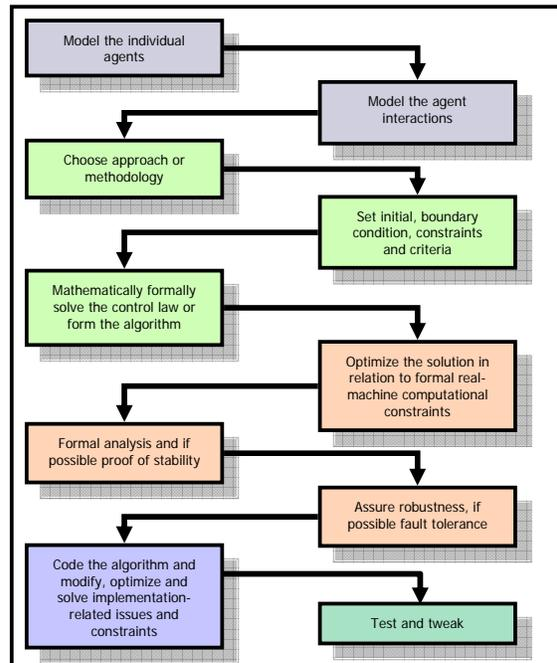
Figure 2: The meta-algorithm that encapsulates the coordinated control paradigm
