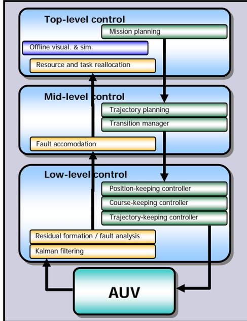
Figure 1: The hierarchical topology of a generalized coordinated control system
