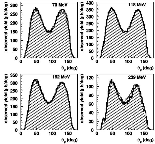
FIG. 2. The polar angle  $\theta$  of the two protons from the selected  $[pp]$  channel in the  $\pi$ - $d$  center-of-mass system. The dark solid line is the data, the hatched histogram the sum of the fitted Monte Carlo distributions. The yields have not been corrected for detector acceptance and losses, nor for the effects of the kinematic cuts applied.
