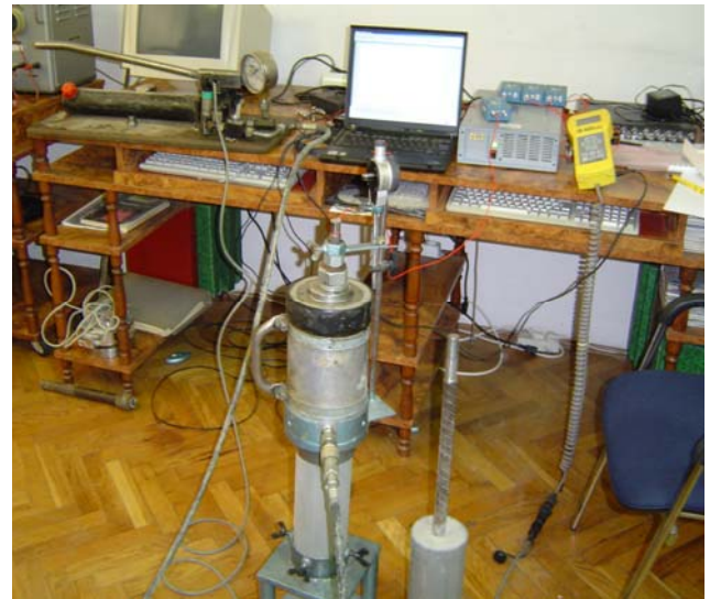
Figure 2. Equipment for pull-out tests with acoustic emission (Arbanas et al., 2005)
