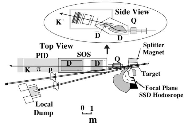
FIG. 3. The experimental plan view showing both the kaon spectrometer (SOS) and the electron spectrometer (ENGE). The SOS is a QDD spectrometer with  $Q$  an entrance quadrupole, and  $DD$  two dipoles bending in opposite directions, providing large momentum acceptance but reducing dispersion.
