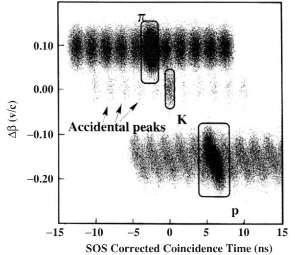
FIG. 4. A plot of SOS particle velocity vs the electron-kaon time-of-flight showing the separation of pions, kaons, and protons.
