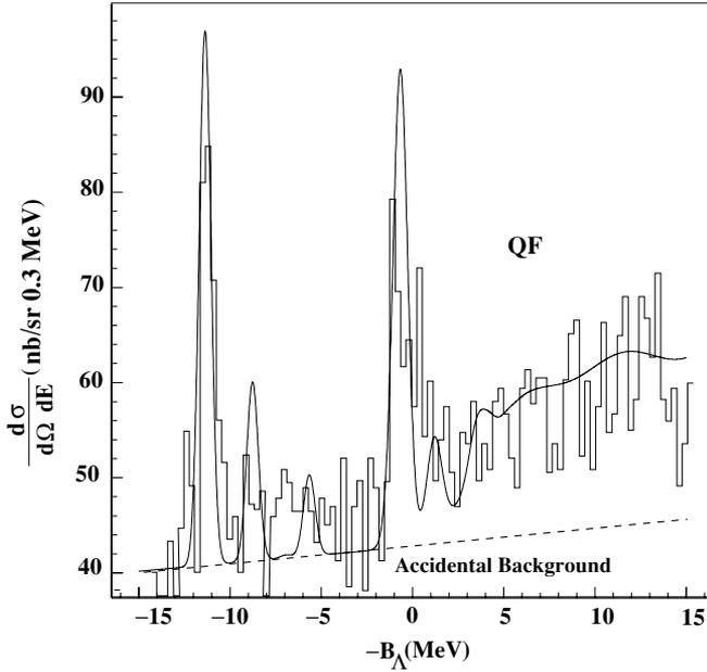
FIG. 7. The binding energy spectrum for  ${}_{\Lambda}^{12}\text{B}$  electroproduced from a C target. The dashed line is a polynomial fit to the measured accidental background, and the curve is a theoretical calculation, spread as described in the text and overlaid on, not fit to, the data. The bin width was 0.3 MeV.
