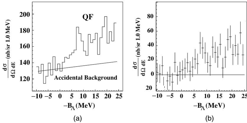
FIG. 10. The binding energy spectrum for  ${}^7_{\Lambda}\text{He}$  electroproduced from a  ${}^7\text{Li}$  target. The data are binned in 1 MeV intervals. In (a) the zero in the cross section scale is suppressed. (b) shows the background subtracted spectrum with statistical errors.
