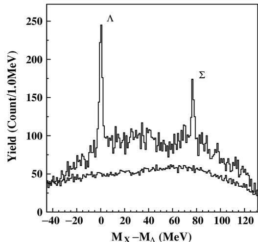
FIG. 6. The missing mass spectrum obtained from a  $\text{CH}_x$  target showing both  $\Lambda$  and  $\Sigma$  production from hydrogen in the target. The solid histogram is the accidental background. The bin width was 1.0 MeV.
