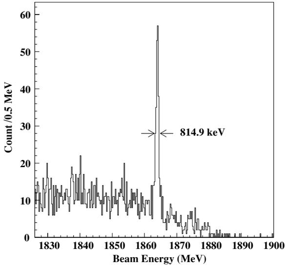
FIG. 5. Reconstructed beam energy from the measurement of Dalitz pairs detected by the spectrometer system. As described in the text, this was used to confirm the energy resolution of the experiment. The bin width is 0.5 MeV.
