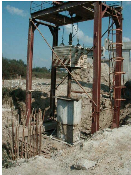
Figure 1: Dynamic testing of piles
