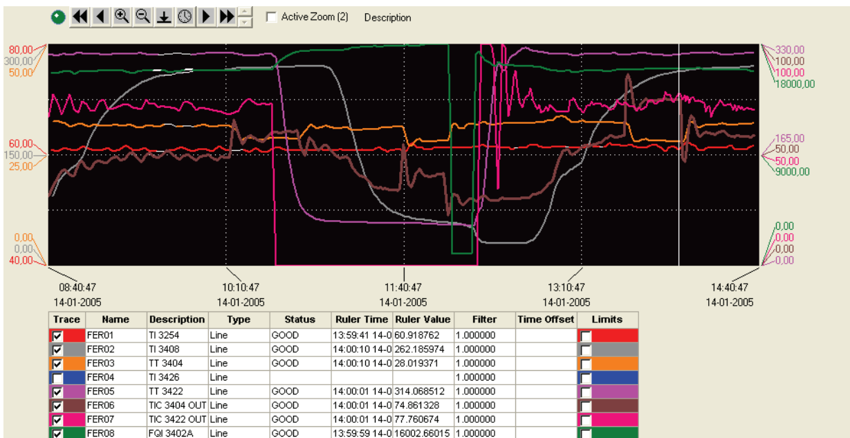
Fig. 4. Process values transient waveforms recorded with mean values of main gas flow 127,149 m 3 /h, outside air temperature 3.9 °C, controller integral time constant T_I = 300 s and controller gain coefficient K_R = 4 - 6 .
