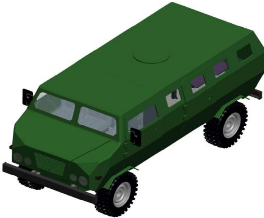
Fig. 1: APV transporter/carrier, countermine and ballistic protection
