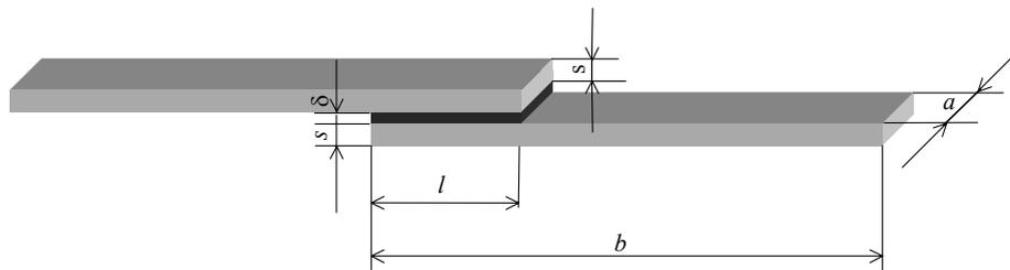
**FIGURE 1.** Geometry of the single-lap adhesive joint.
