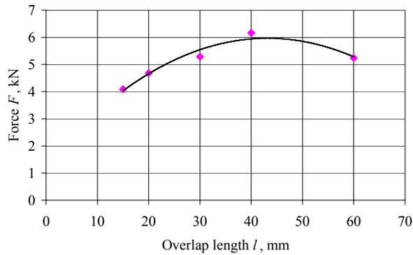
**FIGURE 6.** Joint strength of adhesive lap-joints with different overlap lengths (obtained experimentally)
