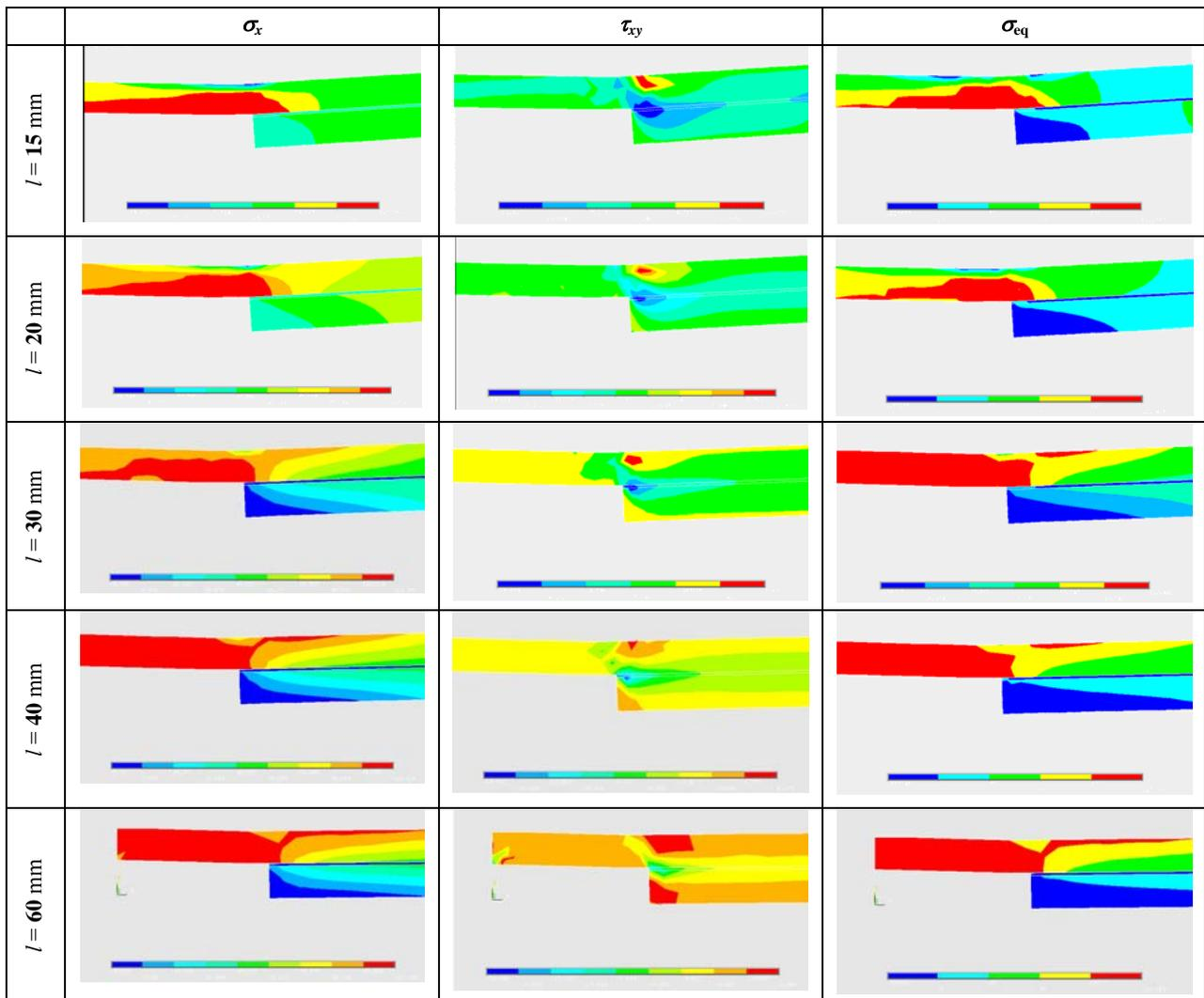
**FIGURE 8.** Axial, shear and equivalent stress distribution in the vicinity of the most critical adhesive joint place.
