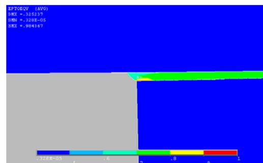
**FIGURE 9.** Total strain enlarged for adhesive material (overlap length is equal to 15 mm).
