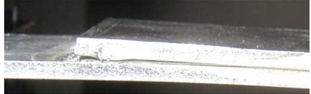
**FIGURE 7.** Failure starts at joint overlap end.
