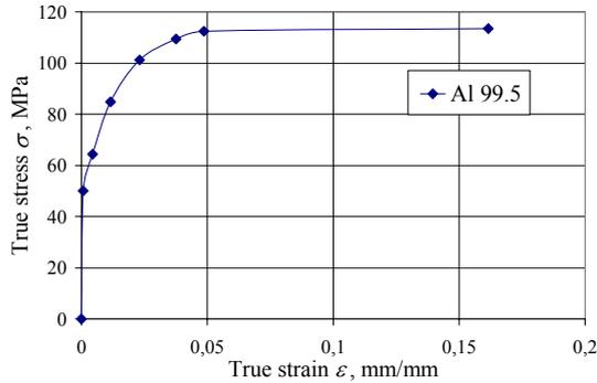
FIGURE 4. Discretized adherend (aluminium) true stress-strain curve used for finite element calculations.
