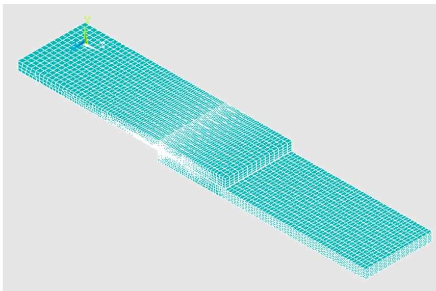
**FIGURE 2.** 3D finite element mesh of the single-lap adhesive joint ( $l=30$  mm).
