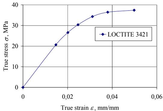
FIGURE 5. Discretized adhesive (epoxy) true stress-strain curve (marked points used for finite element modeling).
