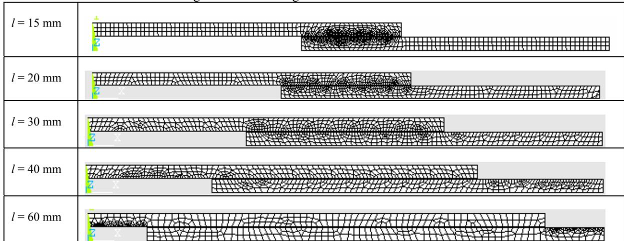
FIGURE 3. Finite element meshes for different geometries of the adhesive joint.
