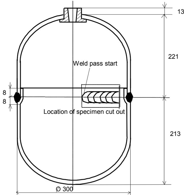
Figure 4. Experimental welding of 1/2 pressure vessel body, and location of hardness specimens cut out
