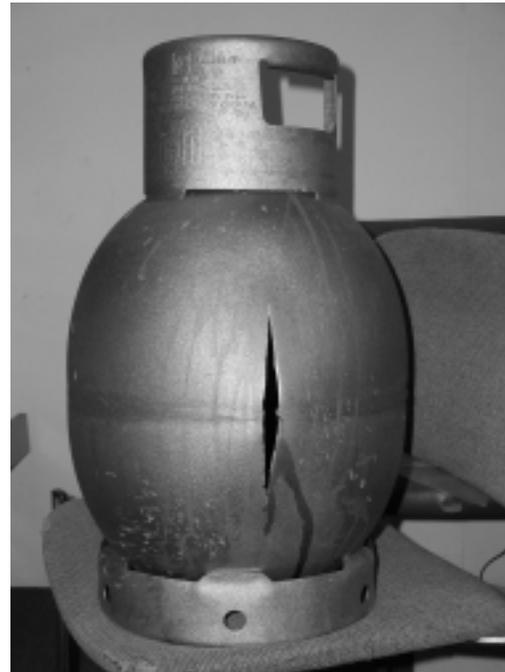
Figure 3. The view of propane/butane pressure vessel (nominal capacity of 10 kg) after pressure test
