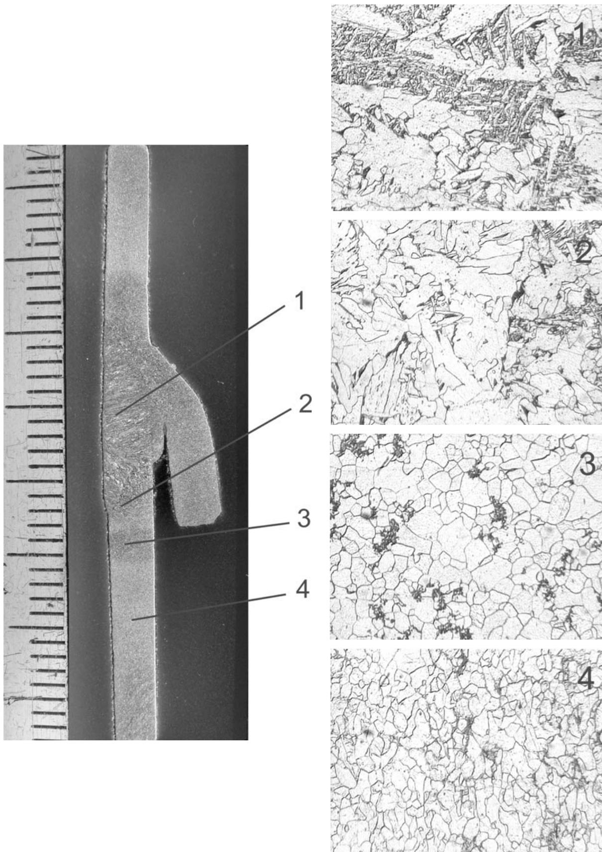
Figure 12. Macro and micro analysis of the welded joint on the weld start
