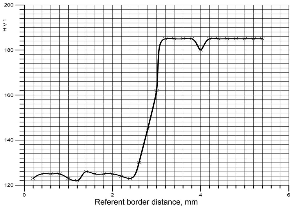
Figure 7. HV1 hardness on the 9,5 mm distance from the weld pass start (line A)
