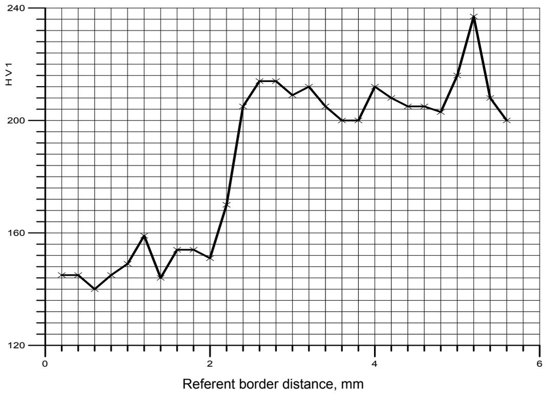
Figure 10. HV1 hardness on the 79 mm distance from the weld pass start (line C)
