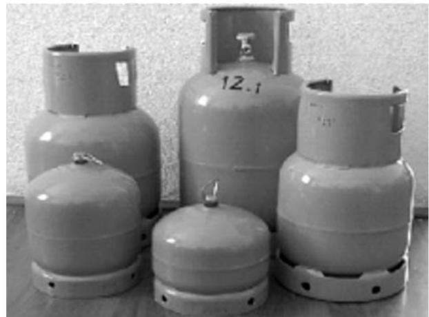
Figure 1. Propane-butane pressure vessels for household with different capacity
