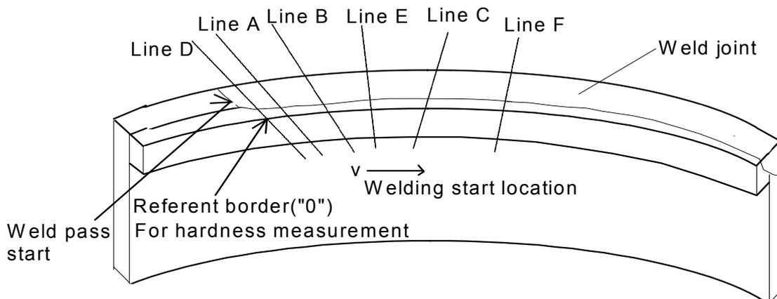
Figure 5. The locations of hardness HV1 measurement on the specimen cut out from the circular pressure vessel weld joint
