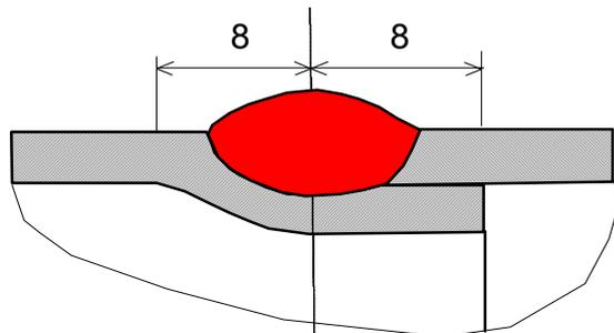
Figure 2. The view of circular weld on pressure vessel body
