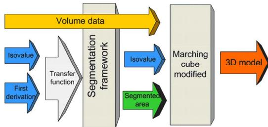
**Figure 5: Segmentation framework and modified marching cube algorithm.**
