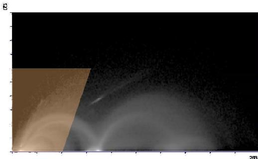
**Figure 6: 2D joint histogram (2D Histogram) of volume data. X axis - intensity level, Y axis - magnitude of first derivative, area presents occurrences  $N(x,y)$  in logarithmic scale. Selected area extracts sinuses and air.**
