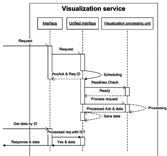
**Figure 3. Client communicates with interface according selected protocol. Requests are unified and sent to unified interface.**
